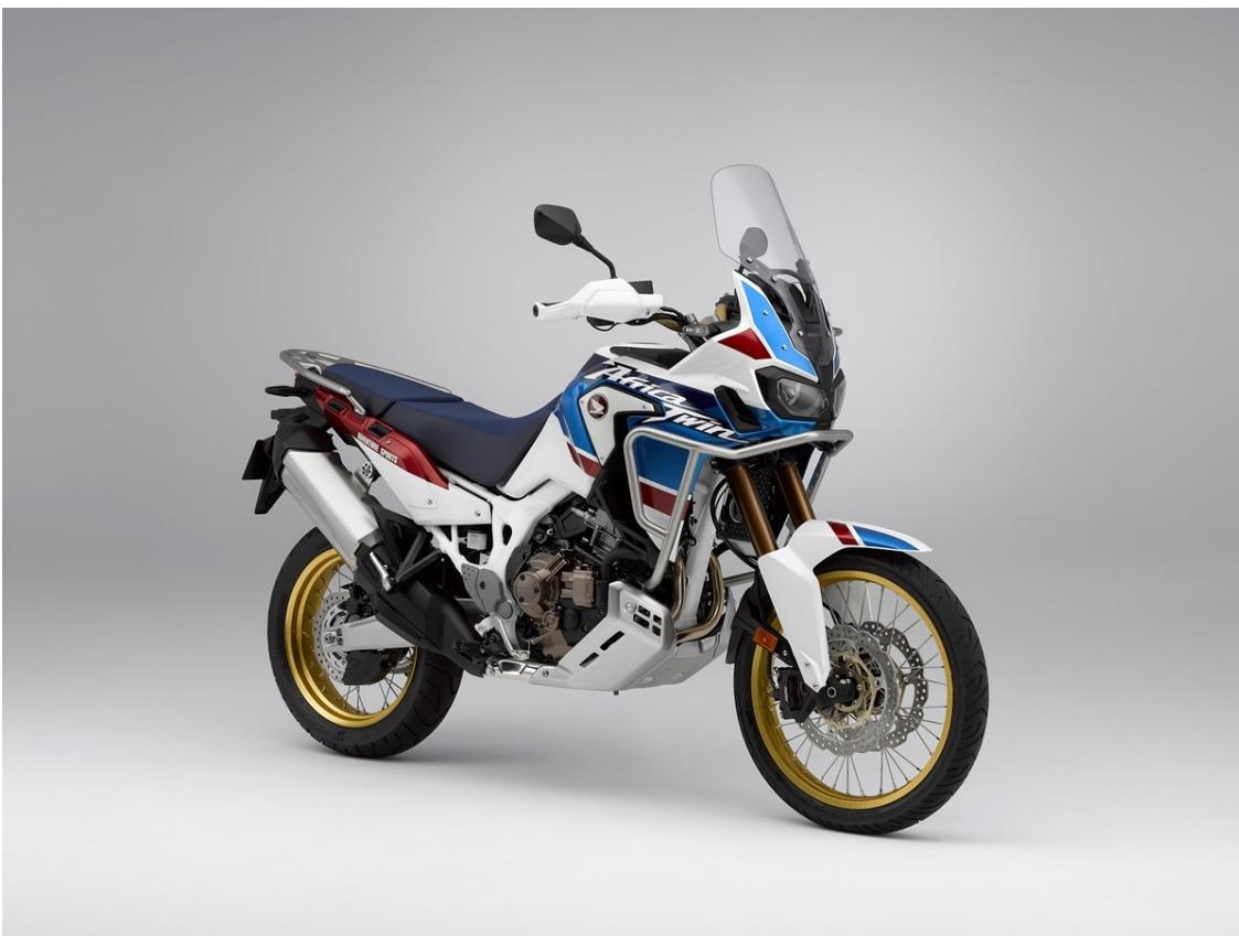
A new version of Honda's definitive full-size adventure machine is ready for Adventure Sports in 2018, with larger fuel tank for a range of over 500km, higher riding position, greater ground clearance, heated grips, extended fairing plus longer travel suspension. It also has Throttle By Wire with 3 riding modes, expanded Honda Selectable Torque Control parameters and revised intake and exhaust. The original Africa Twin's 30th anniversary is celebrated with unique paint scheme.
